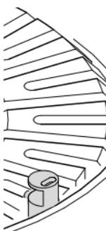
Insert the narrow end of the Occhio tool (supplied) into the groove of the release pin.
