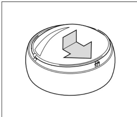
Holding it in this position, clip the edge of the glass insert(s)/lens into the notch on the release pin.
