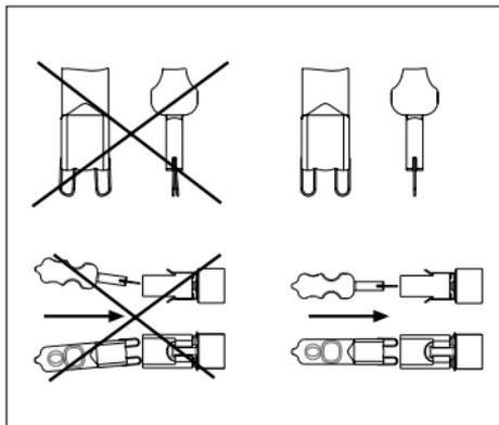
The contacts on the bulb must be aligned in parallel.
