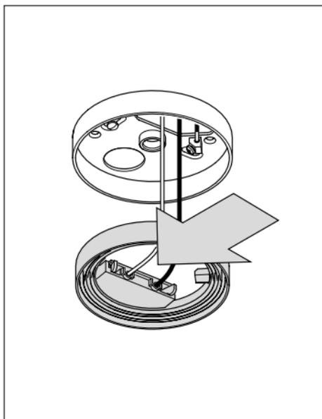
Connect the live and neutral wires to the terminals on the terminal ring.
