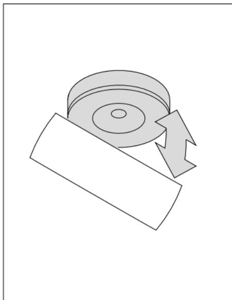
Fold out the base plate with spacing box on the rear of the spotlight.
