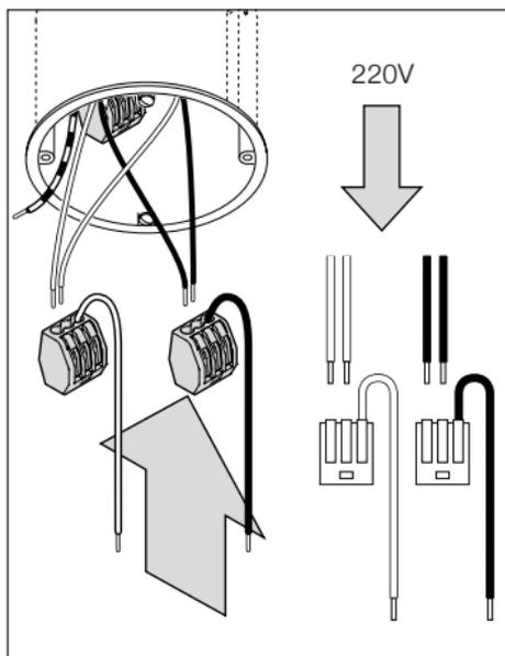
Connect the live and neutral wires to the correct terminals as shown in the wiring diagram.
