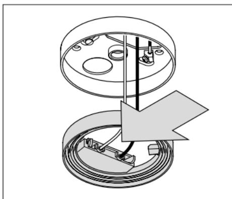
Connect the live and neutral wires to the terminals on the terminal ring.
