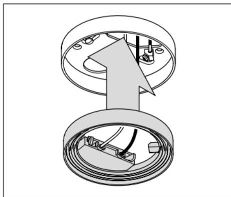
Insert the terminal ring into the spacing box so that ...
