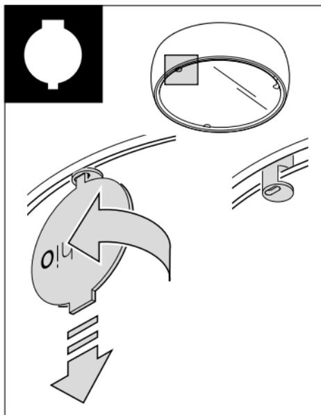
Insert the narrow end of the Occhio tool (supplied) or a screwdriver into the groove of the release pin.
