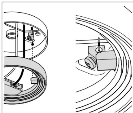
... the earthing terminal is covered by the insulating cap.
