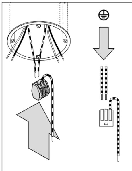
Connect the mains earthing wire to the earthing cable terminal as shown in the wiring diagram.
