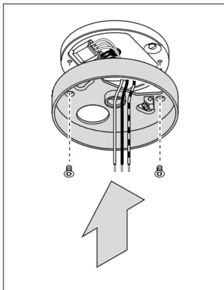
Guide the cable ends for the terminals through the large opening in the spacing box.
