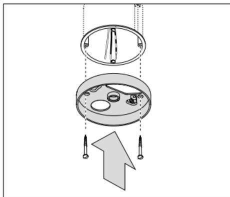
Screw the spacing box directly onto the built-in/plastering box.
