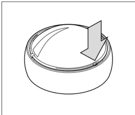
Press the release pin in until it is flush. It clicks into its end position.
