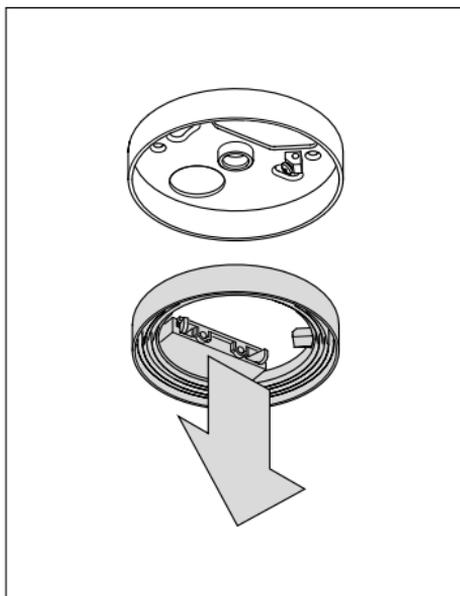
Remove the black terminal ring from the spacing box.
