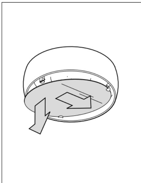
Press the glass insert/lens against the springs and remove from the groove on the release pin.
