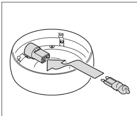
Insert the high-voltage halogen bulb into the G9 pin socket on the head.
