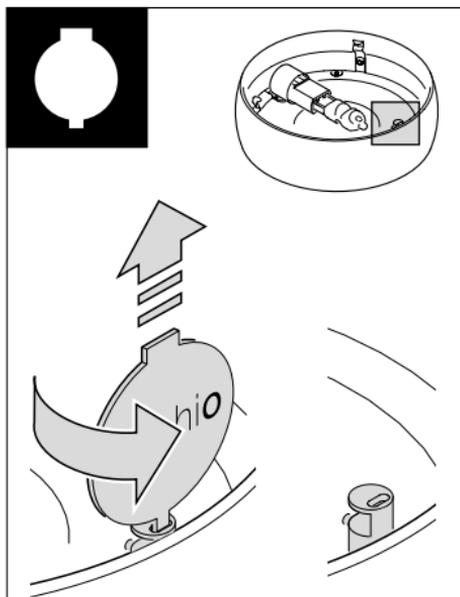
Insert the narrow end of the Occhio tool (supplied) into the groove of the release pin.
