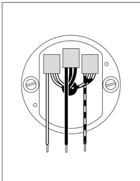
Lay the cables and terminals flush into the opening in the adapter ring.
