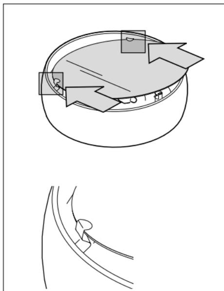
Insert the edge of the glass insert(s) into the two springs and press against the springs.
