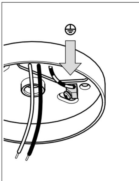
Connect the mains earthing wire to the spacing box terminal as shown in the wiring diagram.
