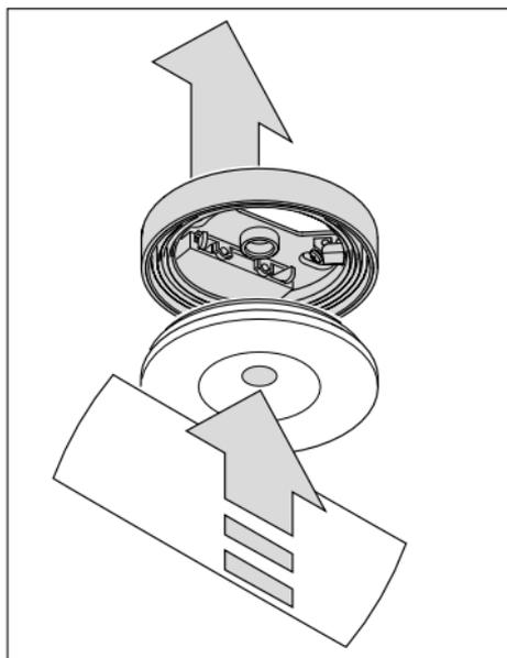
Press the push-button and remove the spacing box from the base plate.
