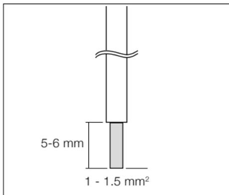
Insulate the ends of the power cables to 5-6 mm.
