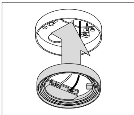
Insert the terminal ring into the spacing
