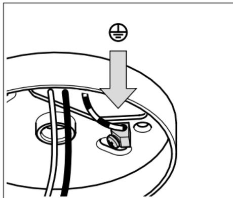
Connect the mains earthing wire to the spacing box terminal as shown in the wiring diagram.
