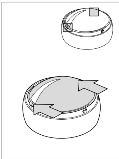
Insert the edge of the lens/colour filter (optional) into the two springs and press against the springs.
