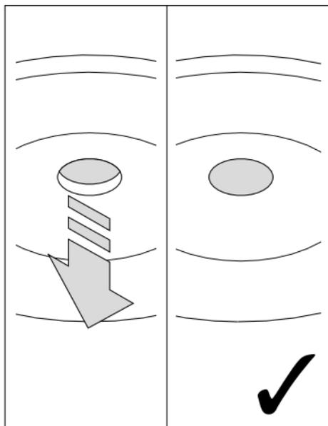
Once the push-button pops out and is flush with the surface and the fastening plate is flush with the spacing box, check that the spotlight is fixed firmly in place by turning/pulling it (see illustration below).
