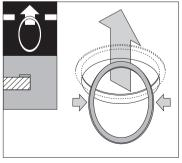
Squeeze the transparent reinforcing rings together slightly, guide them through the openings and place them on the edges of the openings.
