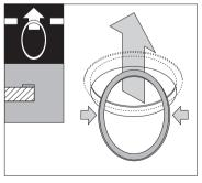
Squeeze the transparent reinforcing ring together slightly, guide it through the opening and place it on the edge of the opening.
