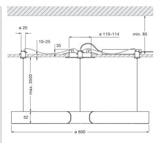
incl. power supply unit (removable) dimensions: L 170 × W 89 × H 27
