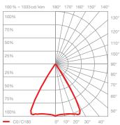
io C with fresnel lens bundled light beam angle approx. 60°
