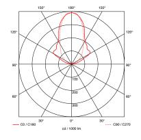
reflector head for light with wide radiation to one side
